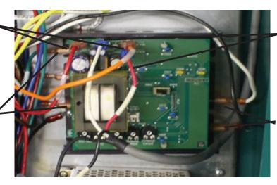
REMOVE THE TWO TRAVERSE SPEED POTENTIOMETER WIRES (1 white and 1 red wire)
