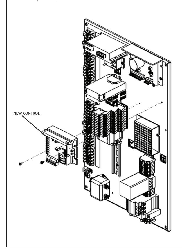
STEP 5: Connect the wires to the new control board as indicated below. Connect the 3 incoming power and 2 output power wires to the new control. Then install the 4 wires included with this kit to S0, S1, S2 and S3 on the new control. Connect the two wires from the traverse speed potentiometer and the other 2 control wires to the 4 wires that were just connected.
