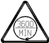
Symbol for caution relating to RPM of the motor and minimum safe rated RPM of the grinding wheel.
