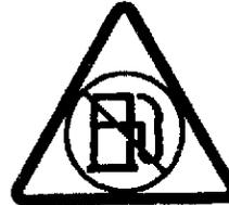
Symbol to keep exposed gasoline or flammables away from the grinder because it operates with a large amount of sparks.
