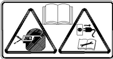
Symbols for Read operators manual, wear safety glasses and disconnect power before servicing.
