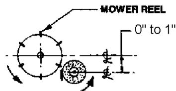
**THE REEL AND GRINDING WHEEL ARE TO ROTATE IN THE SAME DIRECTION.**
