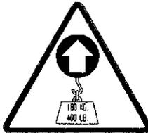
Symbol for maximum weight capacity for winch
