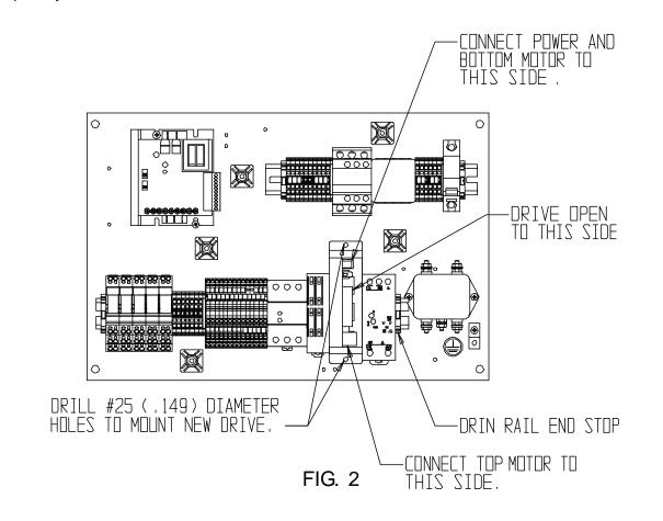
STEP 5: Clean up any debri, then mount the new stepper control to the stepper backet using the 2 socket head screws and nuts. Next, connect the 2 motors, power wires and the control wires to the new Stepper Controller. Reference the Wiring diagrams on the following pages.
