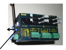
PRY OUT ON BLUE TABS THAT CONNEC TEH PLC TO THE STEPPER. (1 ON EACH SIDE)
